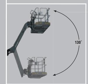
Aichi's articulating jib boom models provide nearly 6-feet of extra horizontal or vertical reach and 130-degrees of working range for increased flexibility.
